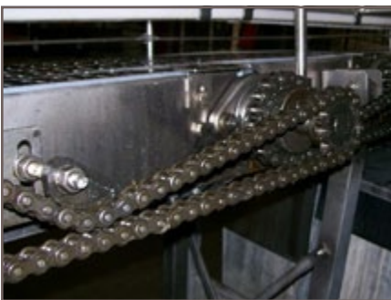
Multi-stage roller chain drives on a conveyor wore unevenly, creating synchronization problems
