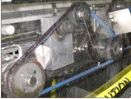
Retrofitting with synchronous belt drives made line speed consistent and eliminated maintenance downtime
